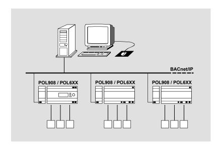
Climatix<sup>™</sup> BACnet/IP communication with POL908.00 Integration guide
